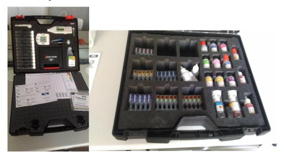
It is a portable photometer to determine concentration of substances in water.
