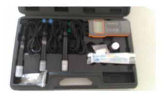
It is a portable device that measure the value of pH, conductivity, salinity and D.O. (Dissolved Oxygen) with automatic compensation of temperature in liquid (fresh and sea water), which had been widely used by Aquaculture, Aquaponics or Fish Farm.
